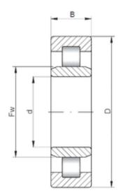
320 mm x 400 mm x 38 mm ISO NU1864 cylindrical roller bearings
