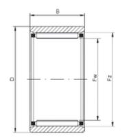
80 mm x 100 mm x 30 mm ISO RNAO80x100x30 cylindrical roller bearings
