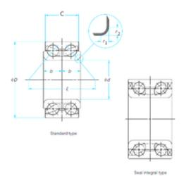
42 mm x 84 mm x 36 mm SKF BA2B444090AB angular contact ball bearings
